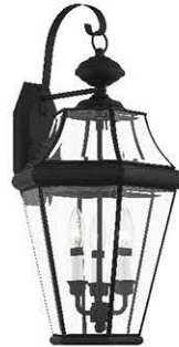
2361-04 LARGE 3-LIGHT WALL LANTERN 12.5" W 24" H 12" EXT BACKPLATE 4.5" W 9" H 1" DEPTH TTM 9.5" H MAX WATT 3 - 60W CAND BASE BULB OPTIONS B10 CA10
